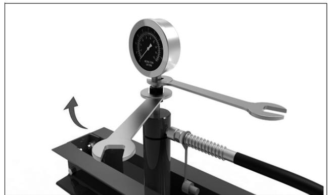
8. Unfasten the protective end cap and screw the hose to the threaded connection of the hydraulic ram.
